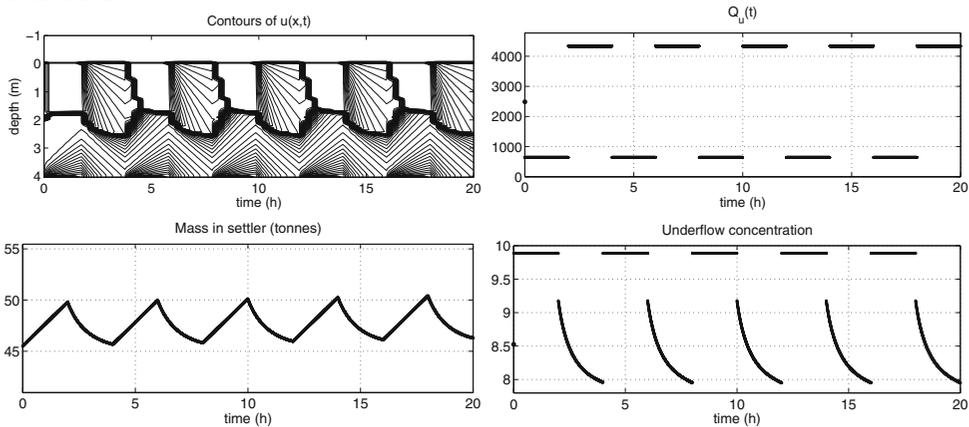
**Fig. 10** Example 2 (continued). A control strategy where  $Q_u^{high}$  is chosen such that  $(u_f, s) \in \mathcal{S}(Q_u^{high})$  during the intervals of high feed concentration, and  $Q_u^{low}$  such that  $\frac{1}{2}(Q_u^{low} + Q_u^{high}) = Q_{u0}$ . Note that the mass is slightly increasing on a four-hour average
