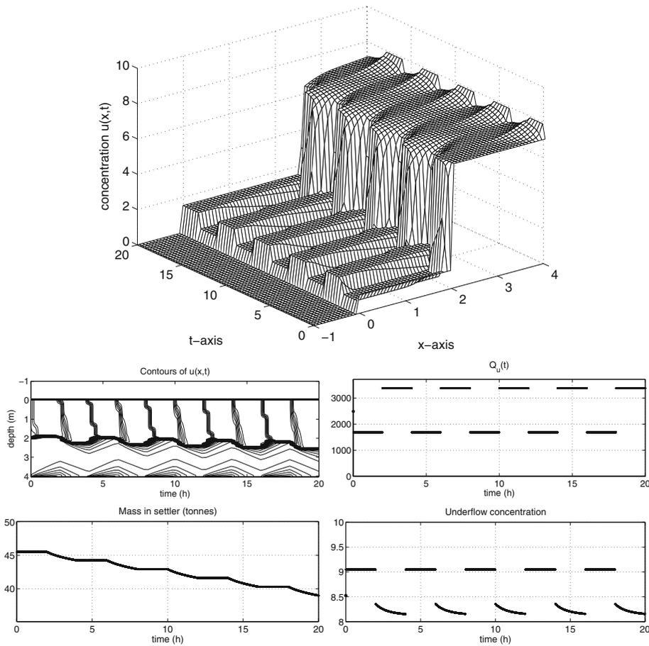
**Fig. 8** *Example 1 (continued)*. A simulation using the same initial data and the same feed concentration as in Fig. 6. DCL1 is applied. The two values of  $Q_u(t)$  are  $Q_u^{\text{low}} = L_1^{-1}(1.8, 5.4) = 1688$  and  $Q_u^{\text{high}} = L_1^{-1}(3.2, 9.6) = 3382$ . Note that the average value of  $Q_u$  is higher than the initial one, which corresponds to a stationary optimal-operation state. Continued simulation shows that the SBL reaches the bottom after 100h
