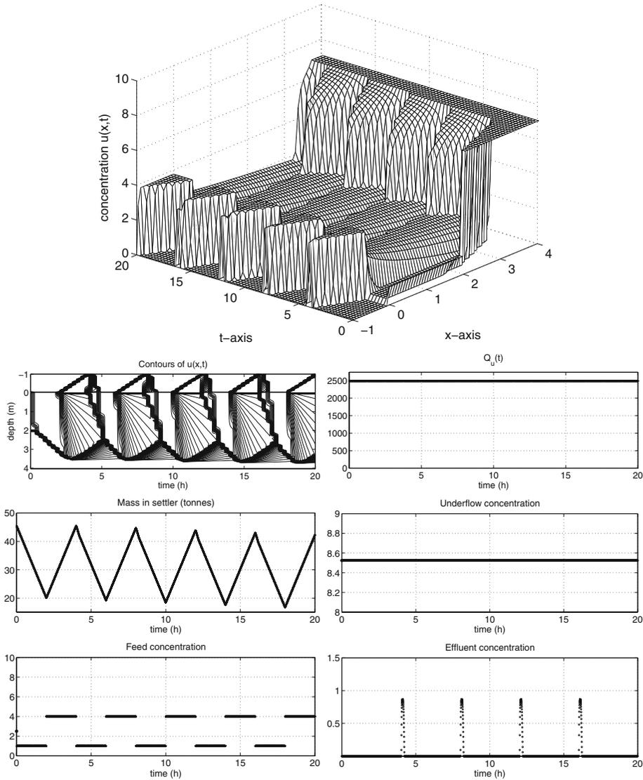
**Fig. 7** Example 2. A simulation where the alternating values of the periodic feed concentration are 1 and 4 kg/m<sup>3</sup>. This larger amplitude than in Example 1 implies overflow and a slightly declining SBL and mass, on an average.  $Q_f(t) = 8482$ ,  $(u_{f0}, s_0) = (2.5, 7.5)$ ,  $u_u(t) = u_{u0} = 8.52$  and  $Q_u(t) = Q_{u0} = L_1^{-1}(u_{f0}, s_0) = 2488$
