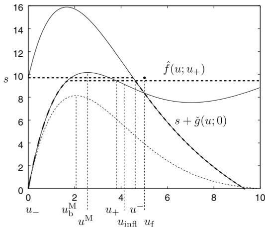
**Fig. 4** A case when optimal operation is not maintained despite  $(u_f, s) \in \mathcal{S}$  and  $Q_u < \bar{Q}_u$ . The concentration value of the maximum of the batch settling flux is denoted by  $u_b^M \equiv u^M(Q_u = 0)$ . Note that  $u_+ = u_+(0)$  is the boundary value below the feed inlet at  $t = 0-$  and  $u^- = u^-(0)$  the new one above the feed inlet at  $t = 0+$ . Since  $u^- > 0$  optimal operation is left
