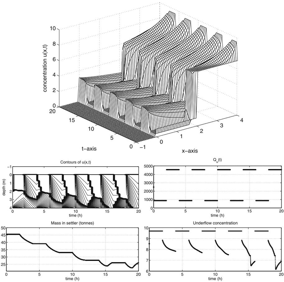
**Fig. 9** Example 2 (continued). A simulation using the same initial data and the same feed concentration as in Fig. 6. DCL1 is applied. The two values of  $Q_u(t)$  are  $Q_u^{low} = L_1^{-1}(1, 3) = 875$  and  $Q_u^{high} = L_1^{-1}(4, 12) = 4563$ . The SBL and mass are declining and optimal operation is left after 15 h
