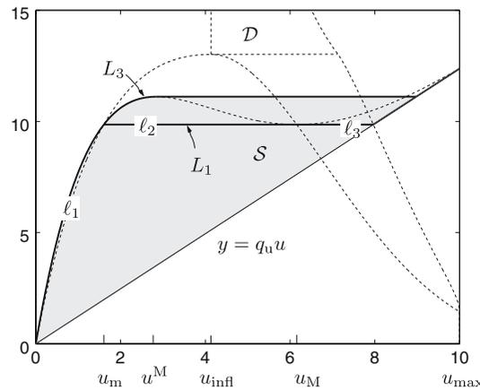
**Fig. 3** The lines  $L_1$  and  $L_3$ , which coincide for low and high concentrations. The set  $S$  (the ‘safe’ region) is the closed region below  $L_3$ , shaded in the figure.  $D$  (the ‘dangerous’ region) is its complement, i.e. it lies strictly above  $L_3$ . (Note that the feed point has to lie on or above the line  $y = q_u u$ , since  $s = Q_f u_f / A \geq Q_u u_f / A = q_u u_f$ .)
