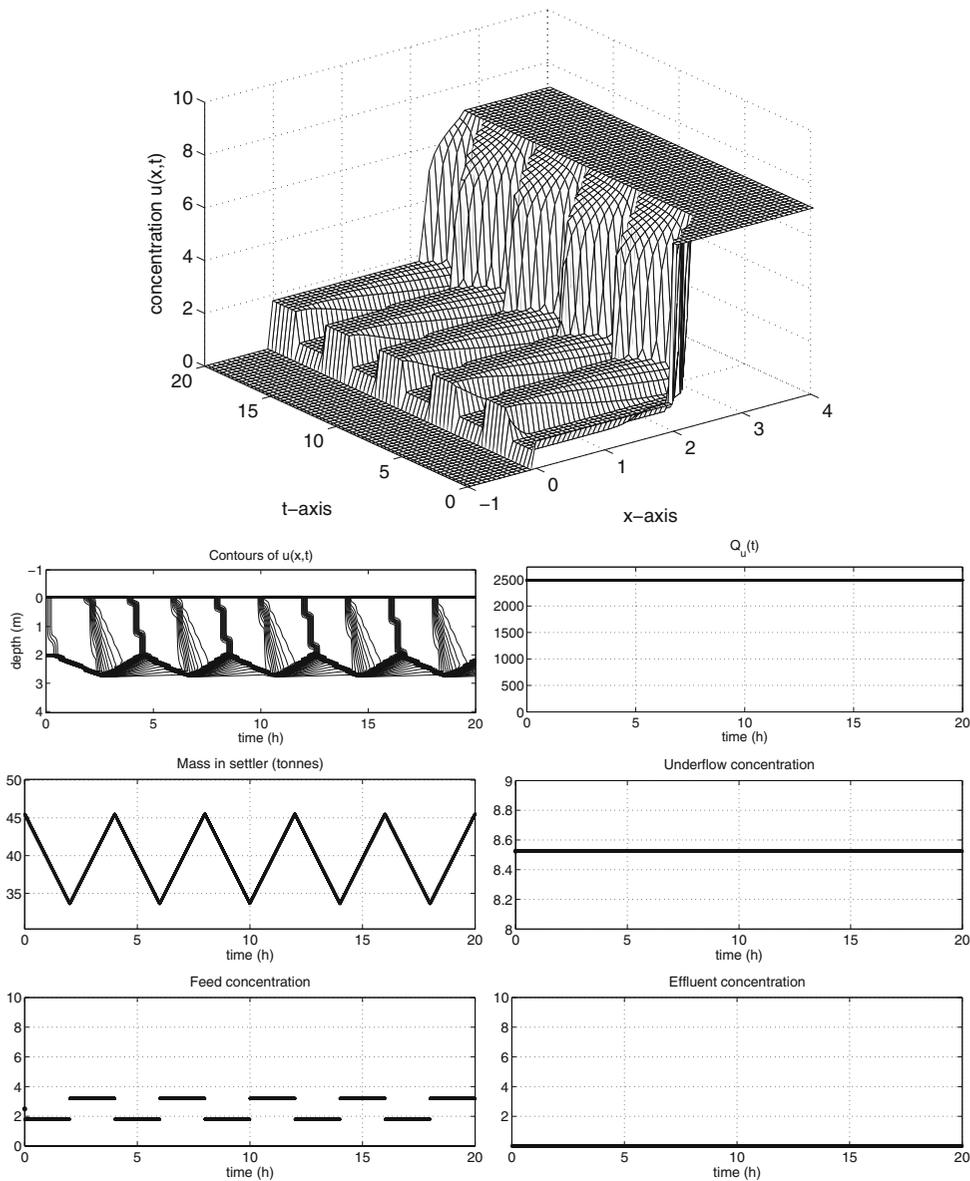
**Fig. 6** Example 1. A numerical simulation as the feed concentration is piecewise constant and periodic with the alternating values 1.8 and 3.2 kg/m<sup>3</sup>.  $Q_f(t) = 8482 \text{ m}^3/\text{h}$ ,  $(u_{f0}, s_0) = (2.5, 7.5)$ ,  $u_u(t) = u_{u0} = 8.52 \text{ kg/m}^3$  and  $Q_u(t) = Q_{u0} = L_1^{-1}(u_{f0}, s_0) = 2488 \text{ m}^3/\text{h}$
